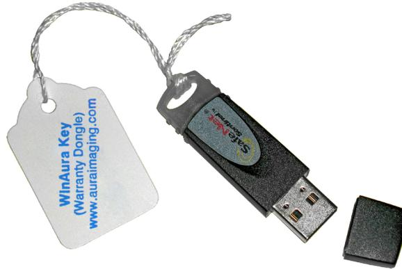
The WinAura Dongle Key can be plugged into any USB port (Figure 2-19). To know if the WinAura Dongle Key has been plugged in and is working properly, a green light on the end of the WinAura Dongle Key will be lit (Figure 2-20).
