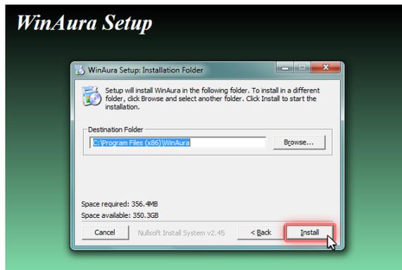
Afterwards, the window “WinAura Setup: Installing” (Figure 2-12) will appear. As WinAura Pro installs, various other windows will appear, such as “TechSmith Screen Capture Codec Installation” and “Sentinel Protection Installer 7.5.0”. All of these are required by WinAura Pro, so simply click on “Install”, “Next”, “OK” and/or “Finish” to continue with the installation.
