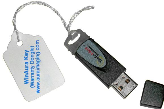
Your copy of WinAura Pro comes with a USB dongle key (Figure 4-1) which allows you to run your copy of WinAura Pro (as well as other WinAura products by Progen/Aura Imaging). WinAura Pro will NOT function if your dongle key is not connected to your computer.
