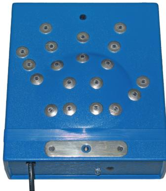
The Aura Sensor Box can be plugged into any USB port (*Figure 2-14*). To know if the Aura Sensor Box has been plugged in and is working properly, a red light on the Aura Sensor Box will be lit (*Figure 2-15*).
